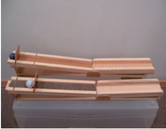
FIGURE 18.2 Ramps context for CVS. A confounded design is illustrated because the ramps differ in ball starting location, type of ball, ramp angle, and ramp surface. (See color plate)
